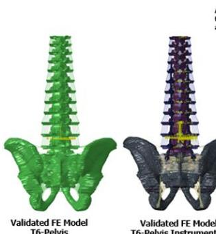
Axial load applied perpendicular to the end plate of T6 Vertebra and 10 mm anterior of its center
